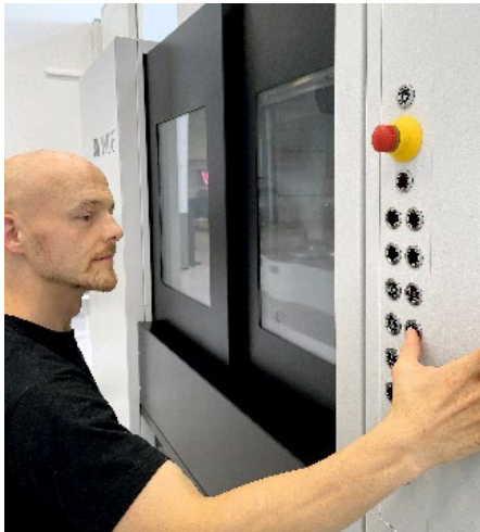
The operating units are used at central access points on the machines to control the workpiece loading or the workpiece loading device.
